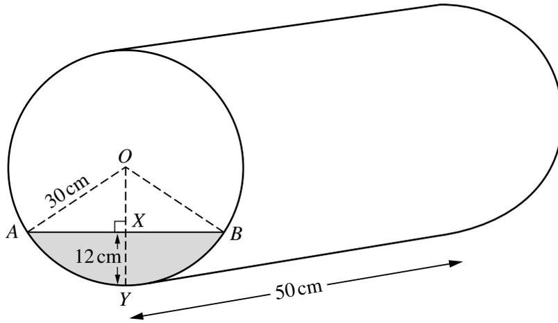
A cylindrical tank, radius 30 cm and length 50 cm, lies on its side.
